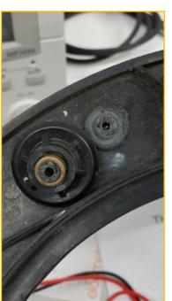
As can be seen in the adjacent photo one of the plastic wheel posts was broken off. The wheels slide over the brass bush and are secured using a pan head screw and large washer.
